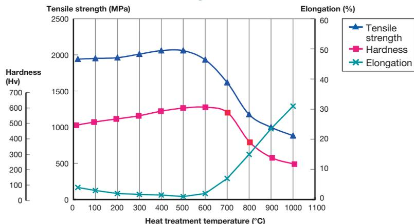
\* The above graph shows the tensile strength, hardness, and elongation when a material with 90% processing rate of wire-drawing is heat-processed at each temperature for two hours.
