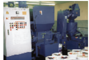
Chip Processor: Separates the oil from the chips and breaks the chips down into small pieces for recycling.
