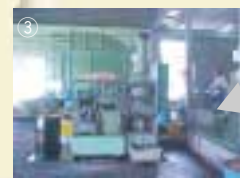
③ The recovered oil is filtered to remove remaining aluminum debris, and the filtered oil is then reused.
