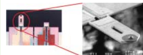
Piezoresistive self-sensitive cantilever: We are aiming to provide a new sensing device, by applying the sensor technology of the piezoresistive self-sensitive cantilever, and the minute pattern forming technology for large difference in steps on the surface, which had been developed for the scanning probe microscope.
