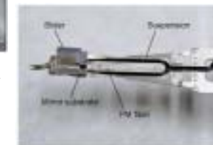
An assembly featuring a near-field light head mounted on a suspension arm and connected to a thin light inducer using fiber optics
