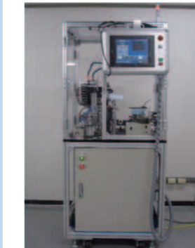
Instrument to measure eccentricity of precision small-bore parts
