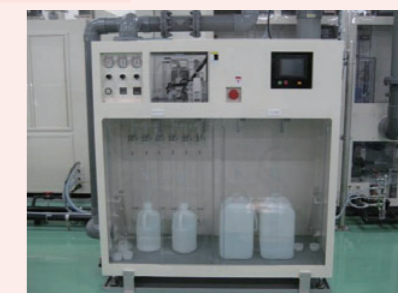
Automatic chemical exchange equipment
