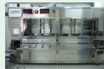
Hydrocarbon cleaning system
