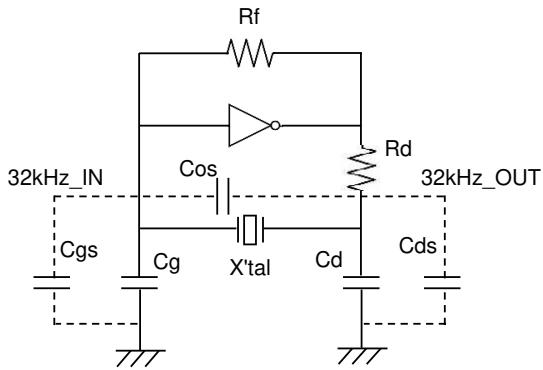
The oscillation circuit has stray capacitance.
