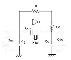
The oscillation circuit has stray capacitance.
