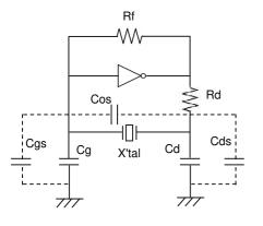
The oscillation circuit has stray capacitance. The CL value is set considering stray capacitance.  $CL = Cg \times Cd / (Cg + Cd) + Cs (pF)$
