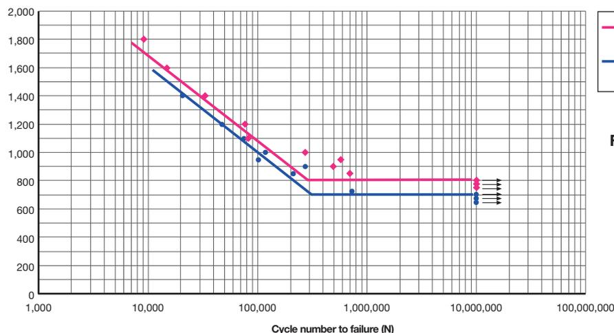
— SPRON100 thickness: 0.130mm (processing rate: 74%, age treatment: 525°C×2h)
