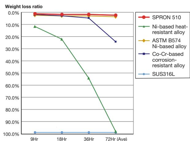
[Measurement conditions] ■ Test piece: φ20mm, Mass 0.2 to 0.3g
