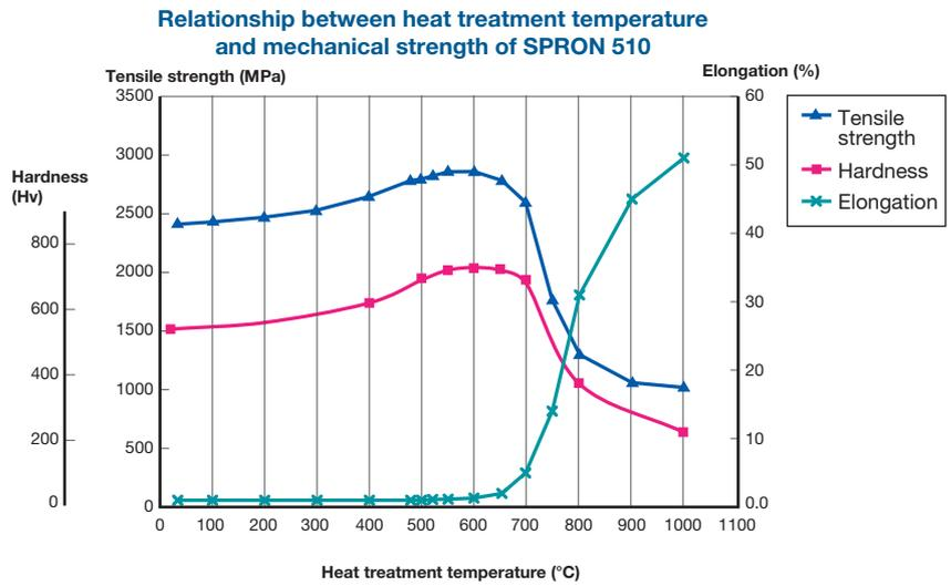
\* The above graph shows the tensile strength, hardness, and elongation when a material with 90% processing rate of wire-drawing is heat-processed at each temperature for two hours.
