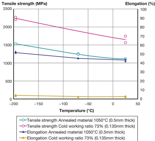
SPRON 510 high temperature tensile testing
