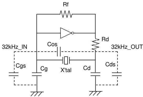
The oscillation circuit has stray capacitance.
