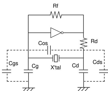
The oscillation circuit has stray capacitance.
