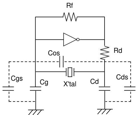
The oscillation circuit has stray capacitance.
