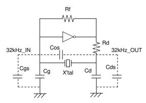
The oscillation circuit has stray capacitance.
