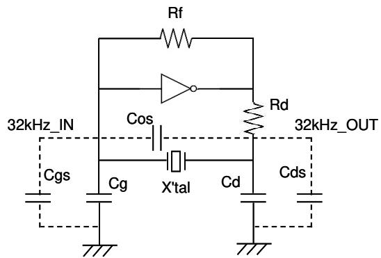
The oscillation circuit has stray capacitance.
