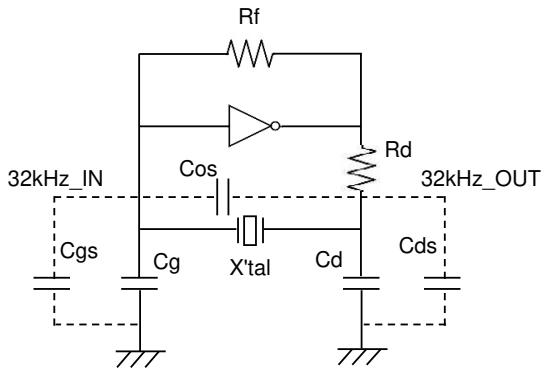
The oscillation circuit has stray capacitance.
