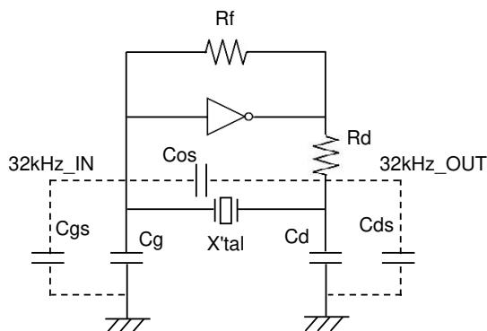
The oscillation circuit has stray capacitance.
