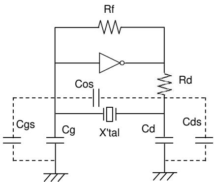
The oscillation circuit has stray capacitance.
