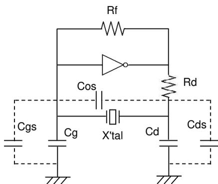
The oscillation circuit has stray capacitance.
