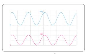
CT-PCB Voltage Output – "V" Version  $\bigcirc$  LUCS DC + 20-kHz sine-wave primary current – i.e.  $I_p[A]$  – and output voltage of a CT-13V version – i.e.  $V_O[V]$
