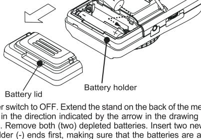
Slide the power switch to OFF. Extend the stand on the back of the metronome. Slide the battery lid in the direction indicated by the arrow to the left, and remove the lid. Remove both (two) depleted batteries. Insert two new batteries into the battery holder (-) ends first, making sure that the batteries are aligned with the polarity markings in the slots. Replace the battery lid. After replacing the batteries, turn the power ON and confirm that the metronome is functioning normally.
